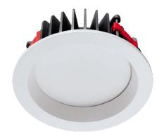
The Sirius IP Mini LED is a 110mm diameter downlight which uses a CREE LED engine. The heatsink is constructed from die-cast aluminium complete with aluminium bezel and reflector.
