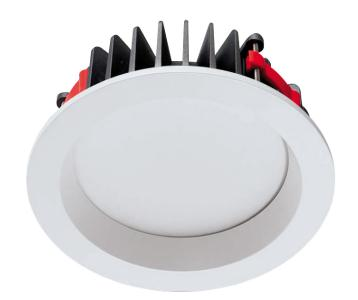
The Sirius IP LED is a 190mm diameter downlight which uses a CREE LED engine. The heatsink is constructed from die-cast aluminium complete with aluminium bezel and reflector.
