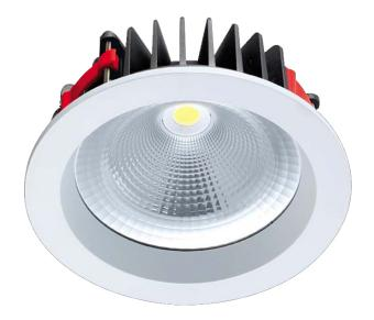
The Sirius LED is a 190mm diameter downlight which uses a CREE LED engine. The heatsink is constructed from die-cast aluminium complete with aluminium bezel and reflector.
