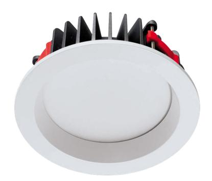
The Sirius IP Max LED is a 230mm diameter downlight which uses a CREE LED engine. The heatsink is constructed from die-cast aluminium complete with aluminium bezel and reflector.
